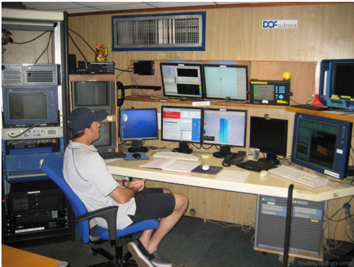
Above photograph shows the navigator's station for operation of the Differential Global Positioning System and Multi-Beam Echo Sounder Systems.
